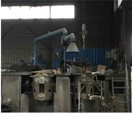
项目熔化炉+可移动集气罩
